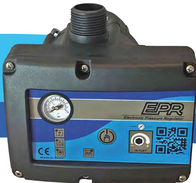
**EPR** - electronic pressure regulator - is an electronic drive for single-phase pumps up to 2,2 kW (1~115-230V) with an innovative system of pressure reduction/regulation in order to mantain an steady outlet pressure.
